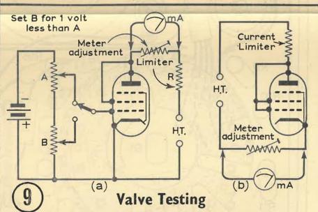
With the aid of the meter, the quality of a valve may be tested. Fig. 9a shows the arrangement for testing mutual conductance. The meter is switched to a suitable current range and indicates anode current. A voltage is applied to the grid, and varied by I volt (this can be done by first measuring the applied voltage, resetting the potentiometer for a 1-volt change, and reconnecting the meter to measure anode current).
