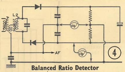
Meter Va is connected across one-half of the resistive load, the secondary L2 detuned and the tuned circuits previous to this adjusted for maximum output. L2 is finally adjusted for balance by applying meter Vb to the centre tap of the load and the centre tap of L2. As the former is at chassis potential and the latter is the a.f. take-off point with respect to d.c., the meter is connected between the a.f. take-off point and chassis. L2 is tuned for null point, zero reading.
