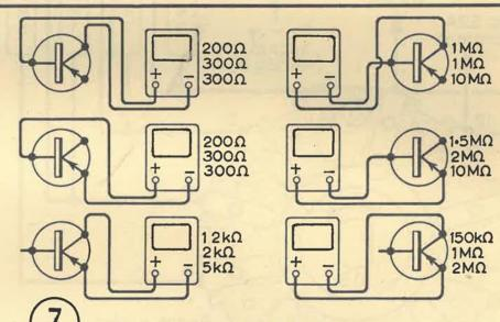
**Transistor Testing** Semiconductors can be checked for back and forward resistance by the application of the ohmmeter in the correct sense (polarity). Remember that the positive terminal presents a negative voltage to the external circuit on the ohms ranges, from the internal battery.
