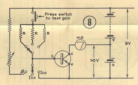
under test is a p-n-p type, connected in the grounded-emitter mode. N-P-N types require potentials of opposite polarity. The three switch positions select collector leakage current (I'co) with base open-circuited, collector current (I'co) at cut-off, with base connected to emitter, and  $\beta$ , current gain.
