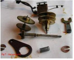
Remove the three wheels that just lift off. The contact fork will just come off as well, with a bit of a wiggle. Remove the clip and spring on the anti-reverse cam (top left Fig 6) being careful to stop the spring doing an impression of Zebedee retiring for the night.
