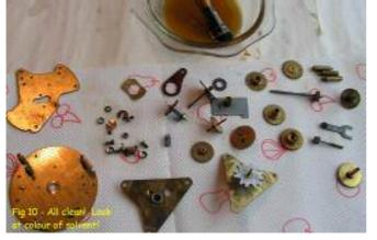
Get a few layers of kitchen paper and lay it out ready. Put each part in solvent, brush it, cleaning all the wheel teeth and pinion leaves, and leave it in the liquid.
