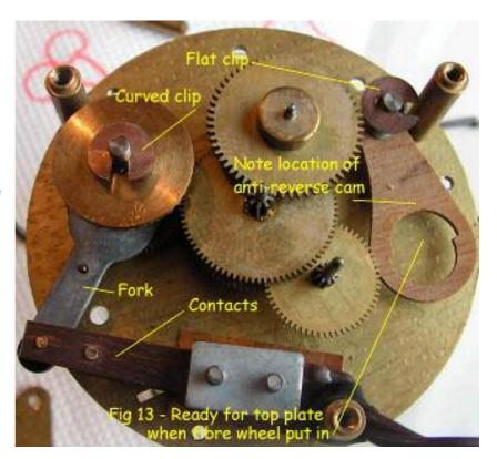
It may be useful to put the pillars in temporarily to hold things together. When everything is in, take any pillars off, and fit the screw that is nearest to the alarm arbor. There may be an earth lead then should be connected to it.
