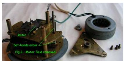
pillars by gripping them with a piece of cardboard or similar, the underside rotor plate will come off. At this point, it is worth taking stock. If the only problem is that the rotor is sticky or noisy, you may get away with no further dismantling.
