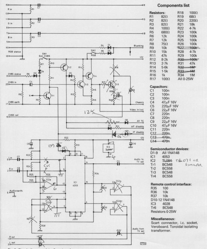
Fig. 3: Circuit diagram of the Scart interface system.
