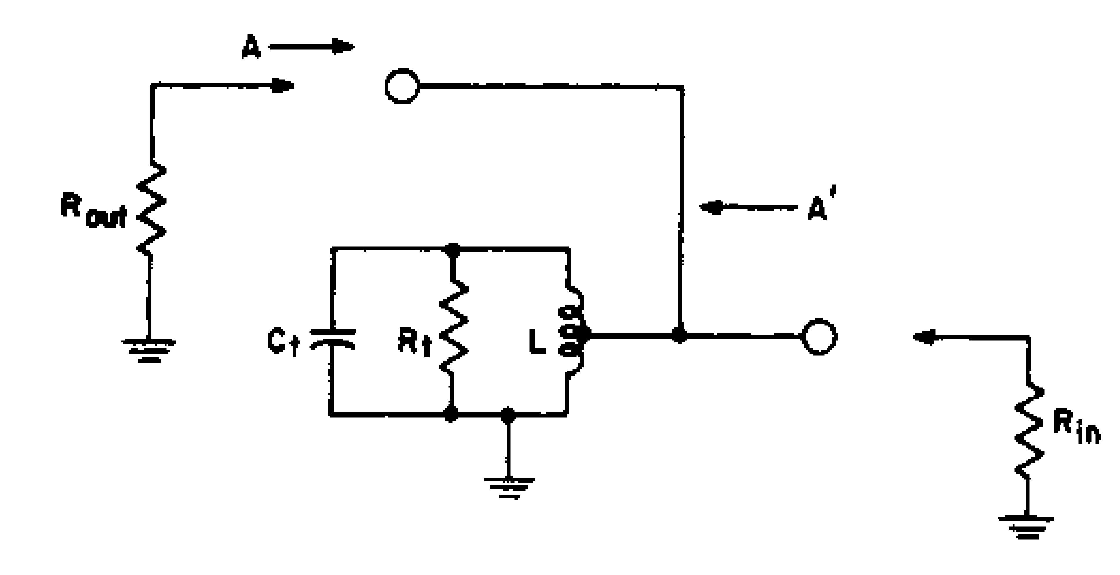
Fig.11 - Equivalent circuit for parallel-tuned circuit.
