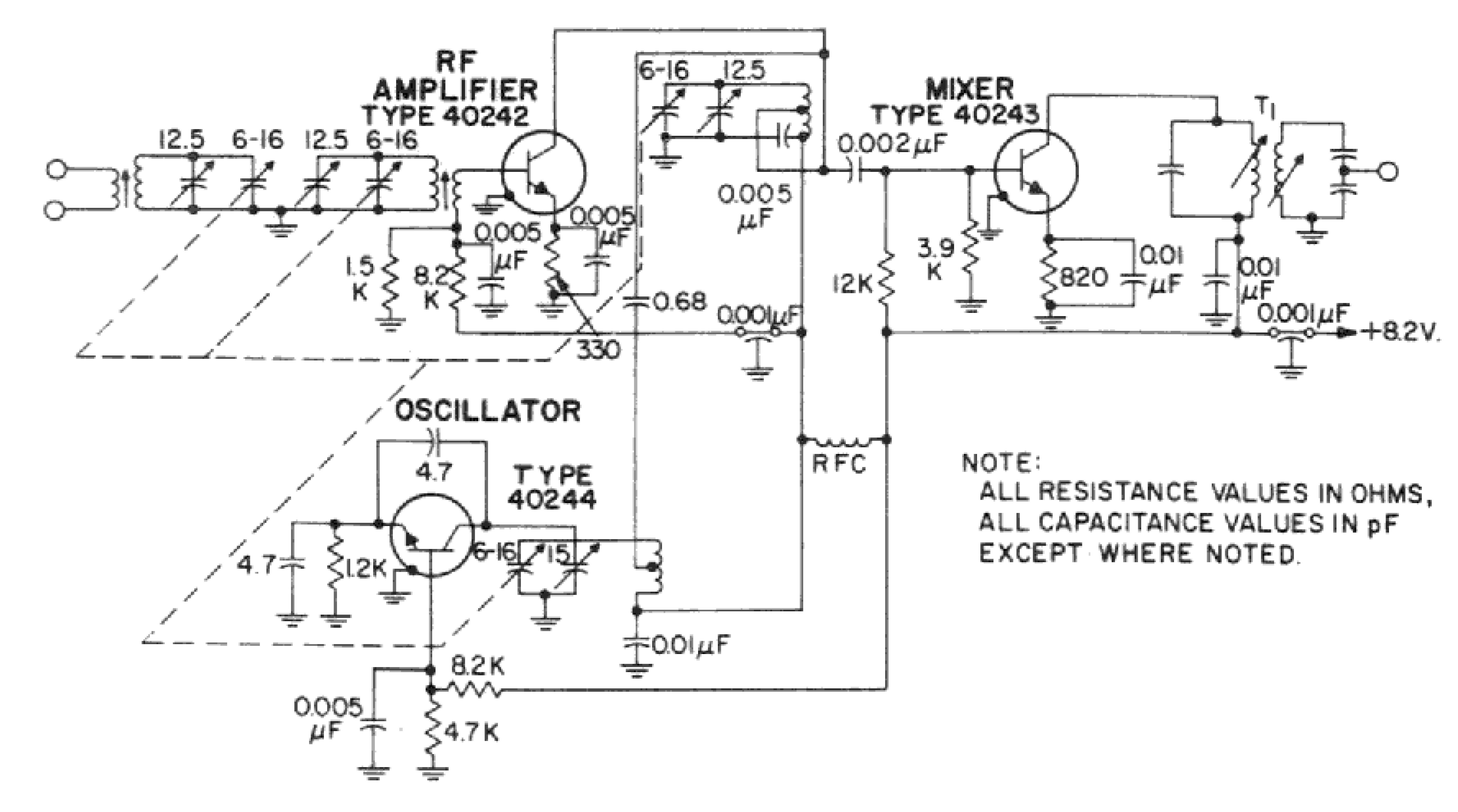
Fig.6 - Circuit diagram of 4-coil FM tuner.
