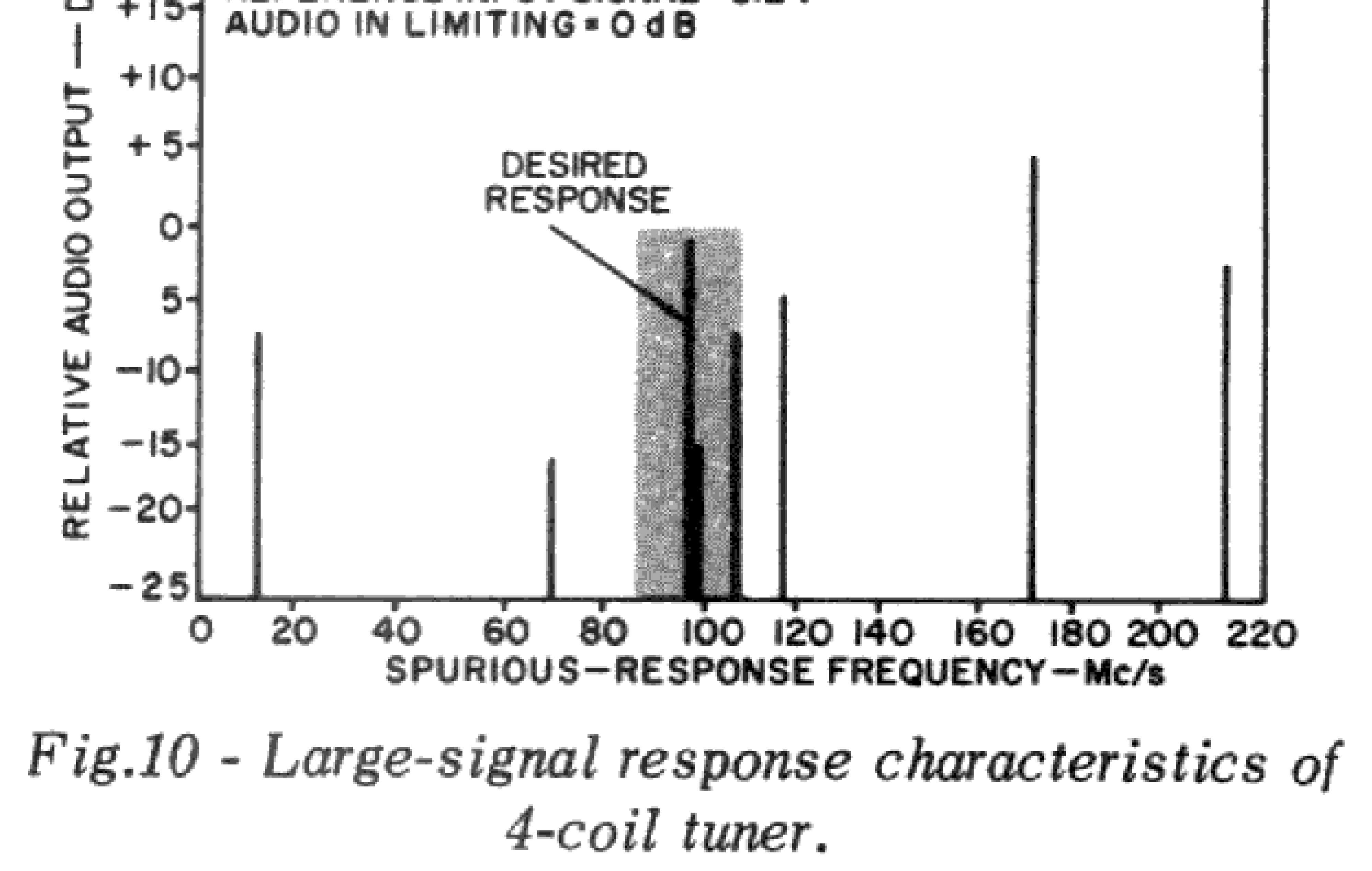
to the tuner. Only two responses occurred in the FM band, with audio output levels 14.5 dB below the reference at 98.7 megacycles per second and 6 dB below the reference at 106.9 megacycles per second.
